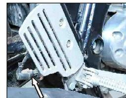
The brake light glows once you press the brake pedal. If brake light is not glowing, check the brake light switch wire for proper connection and the brake light Switch spring for any bend, breakage or disconnection.
