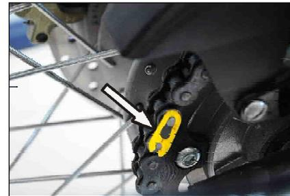
The open end of the chain master link lock should face opposite to normal direction of chain rotation.
