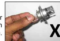
Always hold the bulb with paper or clean dry cloth during handling as shown in fig.
