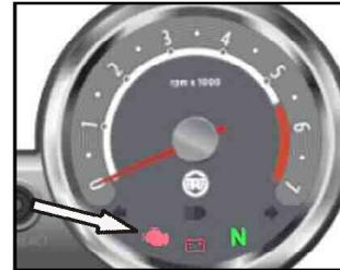
A Malfunctioning Indicator Lamp (MIL) is provided in the RPM meter which is located on the right side of the Cluster unit.
