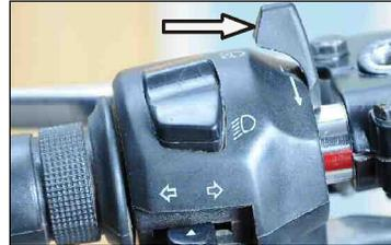
Apply choke in cold start condition while starting the Bike
